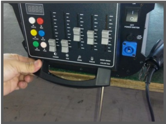
1. Remove the rear handle
